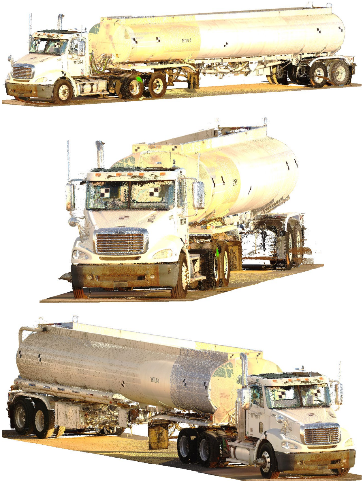
Figure 5.12 Images of 3D Point Clouds of Test Vehicle, Test No. MTL6-1
