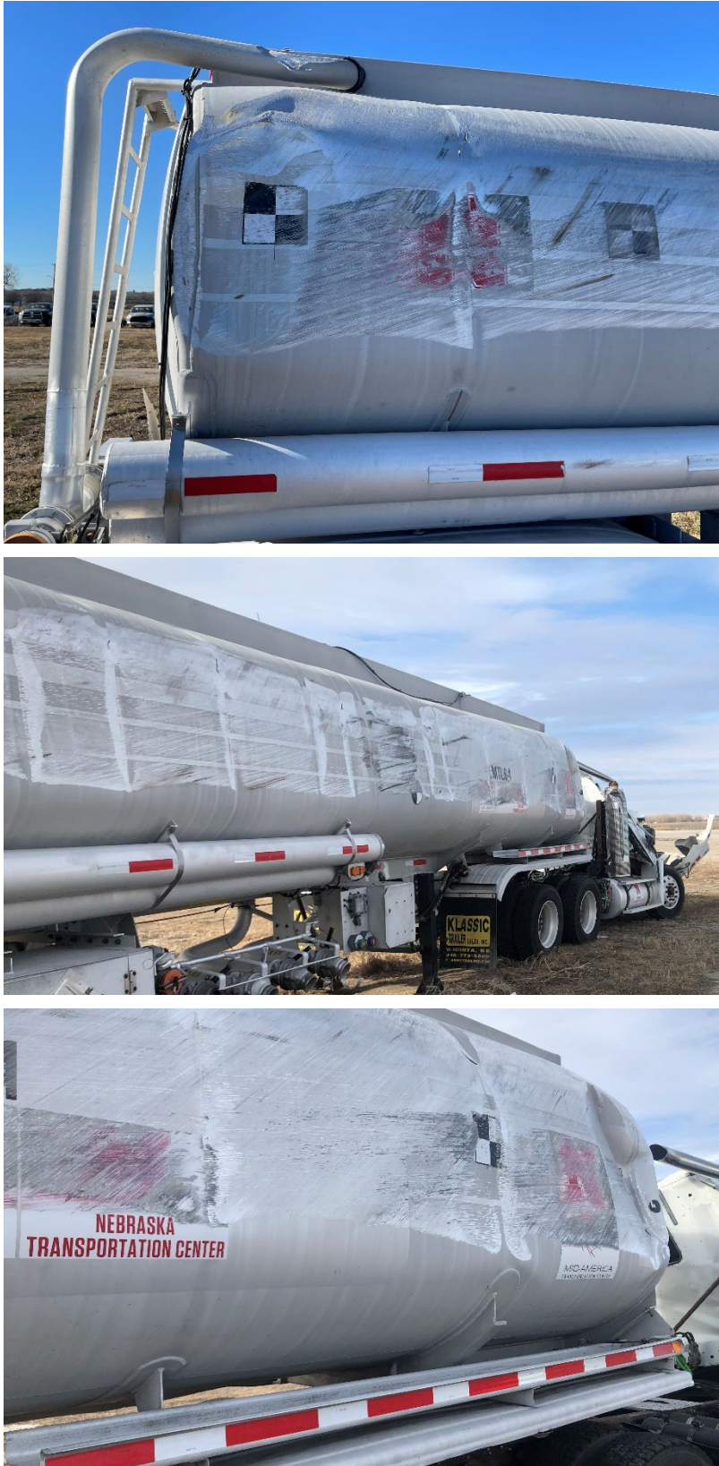
Figure 6.28 Trailer Damage on Non-Impact Side After Being Uprighted, Test No. MTL6-1
