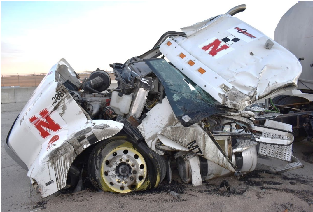
Figure 6.19 Tractor Damage, Test No. MTL6-1 99
