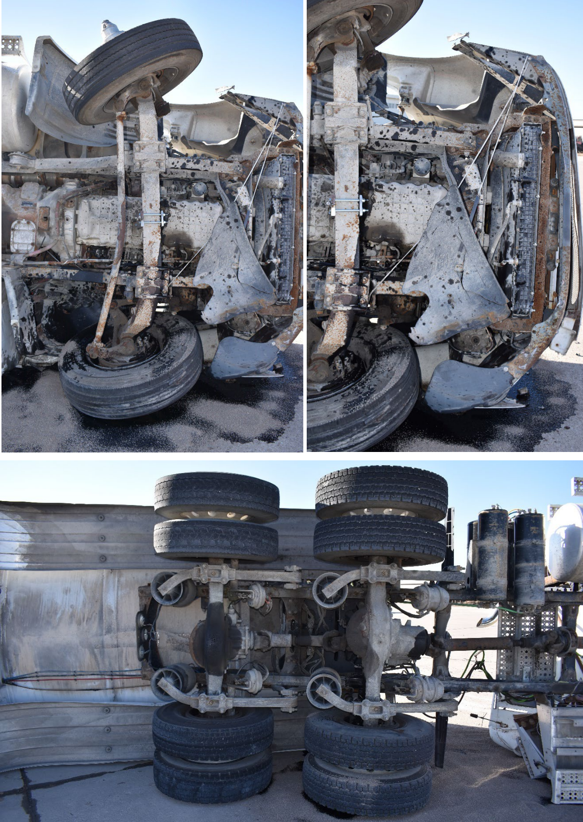
Figure 6.21 Tractor Suspension Damage, Test No. MTL6-1
