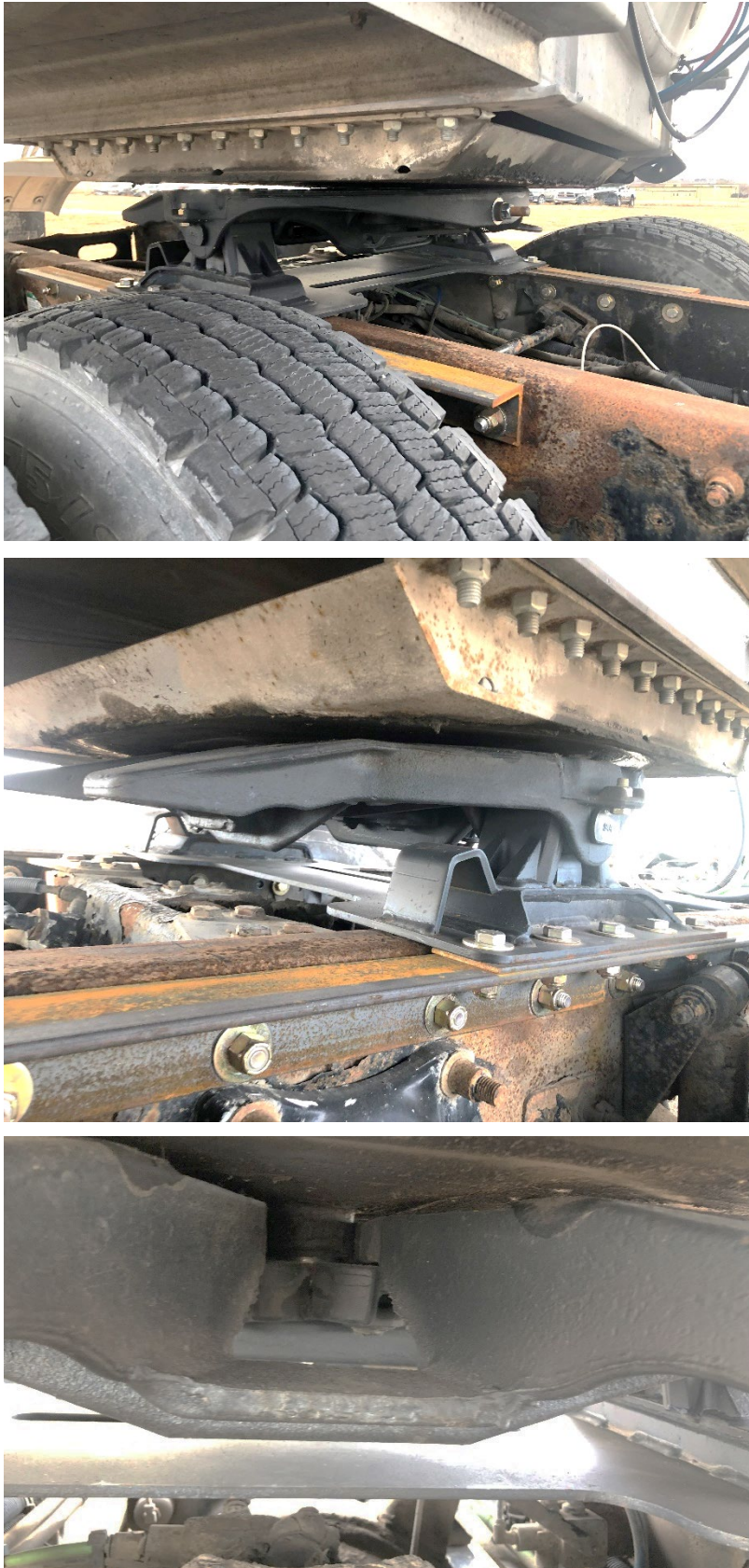
Figure 6.30 Fifth Wheel Damage, Test No. MTL6-1
