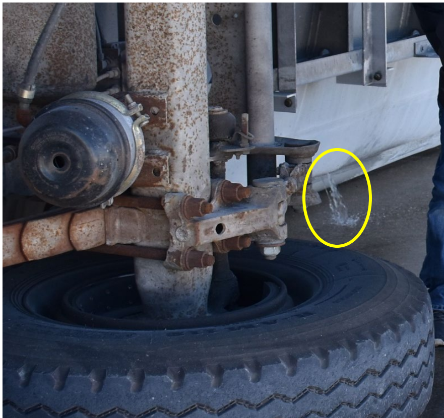
Figure 6.24 Locations of Trailer Leaks, Test No. MTL6-1
